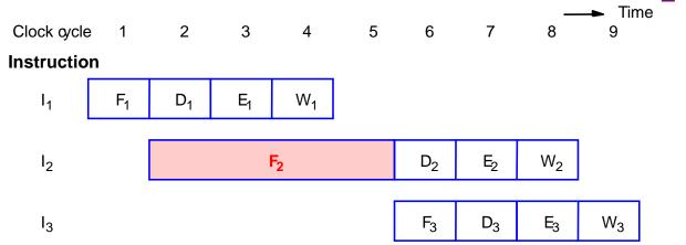
Figure: Instruction execution steps in successive clock cycles.
