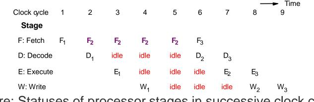
Figure: Statuses of processor stages in successive clock cycles.
